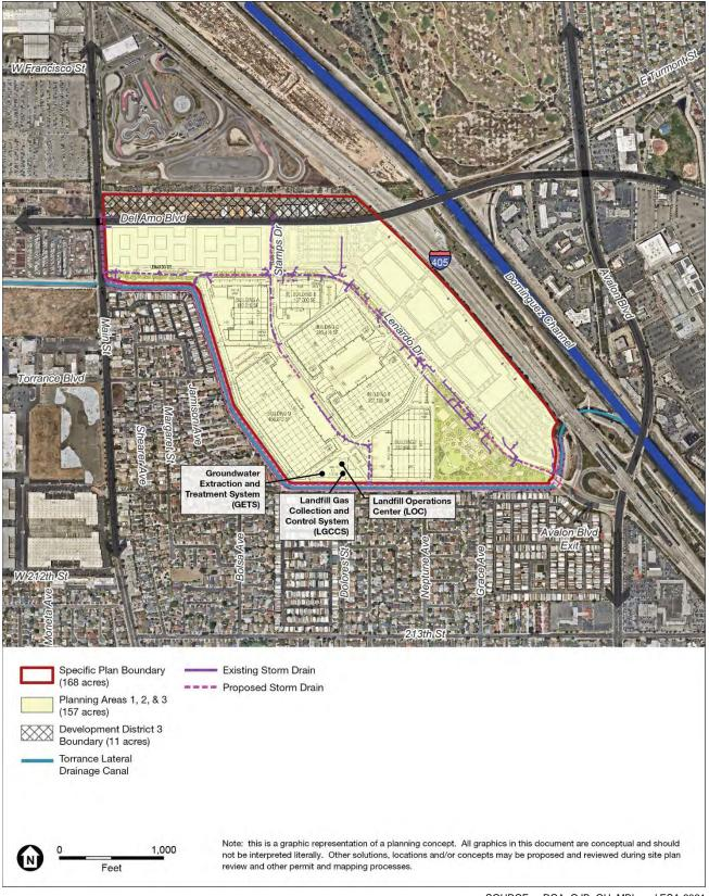
Figure 5.16 Storm Drainage Concept
