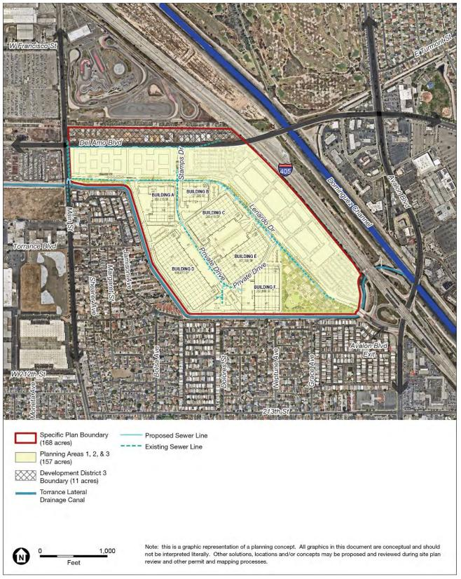
Figure 5.18 Sanitary Sewer Concept
