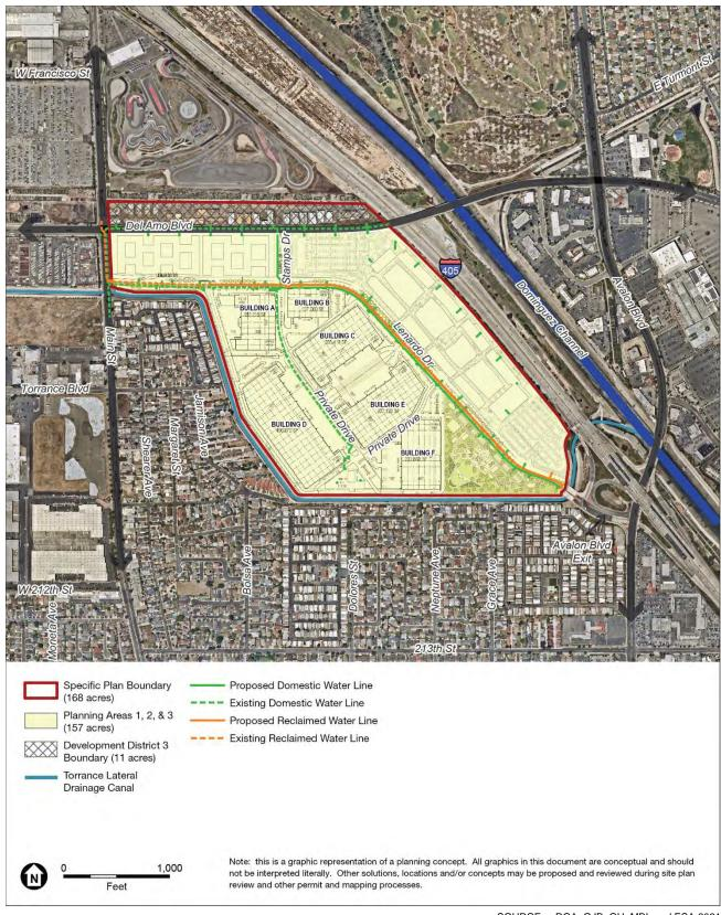
Figure 5.17 Domestic and Reclaimed Water Concept
